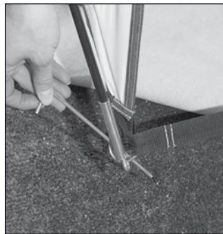
7. If using outside in the grass, stake down the shelter by pushing stakes through the loops and corners at base of shelter.
